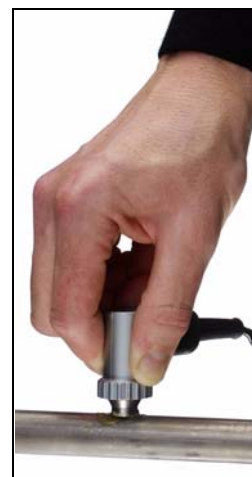
Wall thickness measurement
